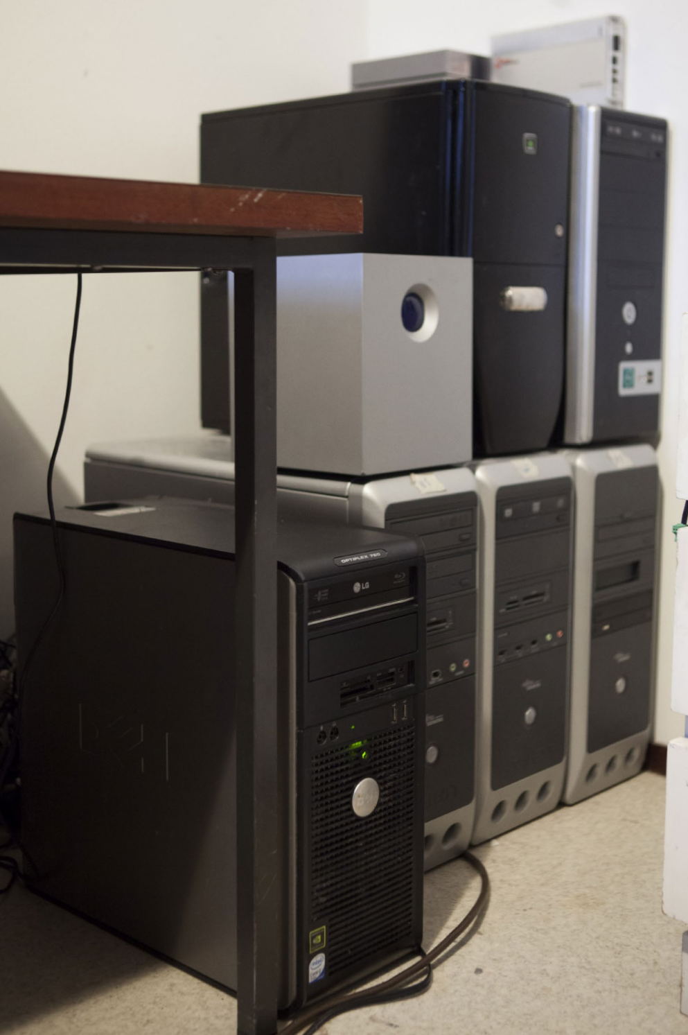
A server farm made of salvaged hardware. Yesterday's powerful PCs work well as a team. The workstation has a RAID disk server connected over eSATA.
